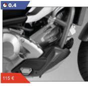
Lower mount shields deflect wind from rider's feet; finished in Black. For DCT model.
