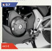
Adjustable ride-by-wire shift lever operated by left foot. Mechanics and electrics pre-set for easy installation.
