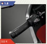
Slim-profile heated grips featuring integrated control with three settings, 'smart' heat allocation that focuses on the hand area most cold-sensitive and battery-drain protection. Heated grip attachment (08T70-MJL-D30) and quartet harness (08A70-MGS-D30) are required to fit this accessory, special heat resistant glue (08CRDHGC-20GMA) is also available.
