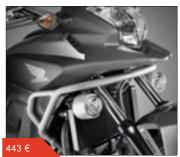
Attachment required for mounting LED fog lights. Cowl ornament (08P70-MGS-D31) is required to fit this accessory.
